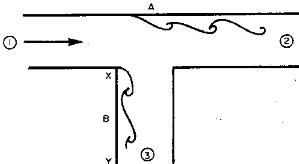
Assuming equal sized pipes, as fluid is removed, the velocities at 2 and 3 are smaller than at 1, the entrance to the tee. Thus the pressure at 2 and 3 are higher than at 1. These two adverse pressure gradients can cause the two separations shown in the diagram above.
