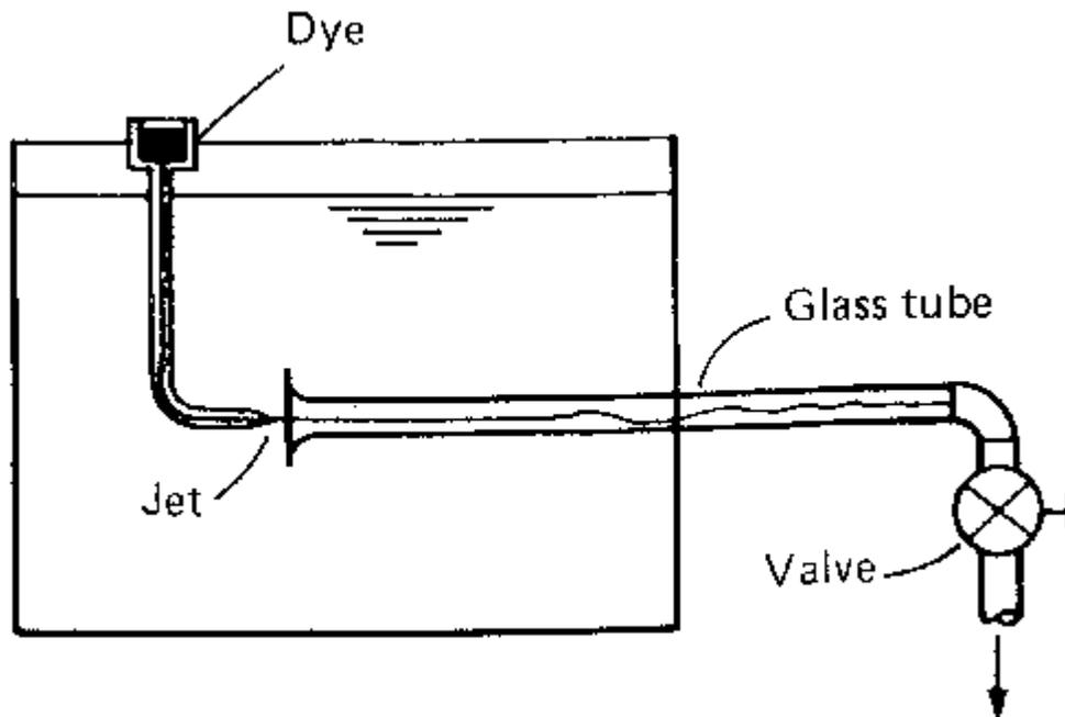
He used a tank arranged as above with a pipe taking water from the centre into which he injected a dye through a needle. After many experiments he saw that this expression
