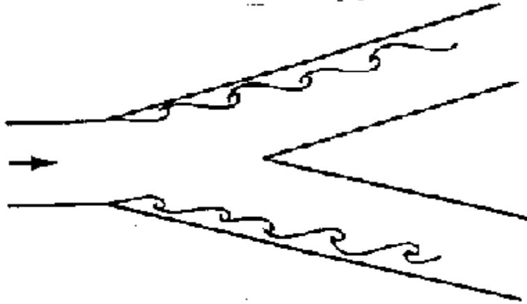
Downstream, away from the junction, the boundary layer reattaches and normal flow occurs i.e. the effect of the boundary layer separation is only local. Nevertheless fluid downstream of the junction will have lost energy.
