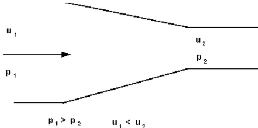
The accelerating fluid maintains the fluid close to the wall in motion. Hence the flow remains stable and turbulence reduces. Boundary layer separation does not occur.
