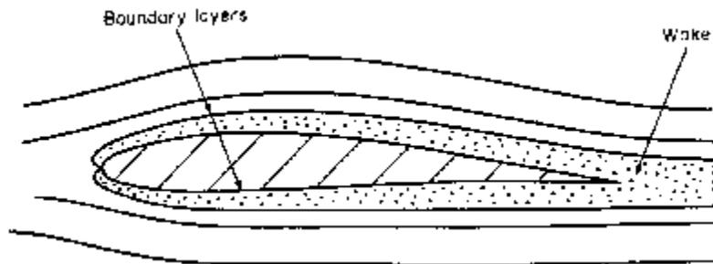
The velocity increases as air flows over the wing. The pressure distribution is similar to that shown below so transverse lift force occurs.
