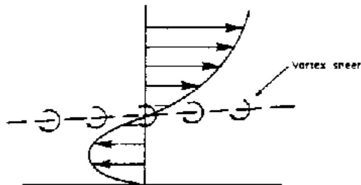
This boundary layer separation and increase in the turbulence because of the vortices results in very large energy losses in the flow.
