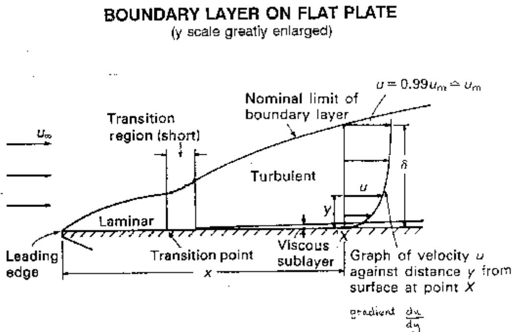
We define the thickness of this boundary layer as the distance from the wall to the point where the velocity is 99% of the "free stream" velocity, the velocity in the middle of the pipe or river.
