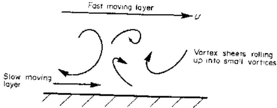
This causes the fluid motion to rapidly become turbulent. Fluid from the fast moving region moves to the slower zone transferring momentum and thus maintaining the fluid by the wall in motion. Conversely, slow moving fluid moves to the faster moving region slowing it down. The net effect is an increase in momentum in the boundary layer. We call the part of the boundary layer the turbulent boundary layer.
