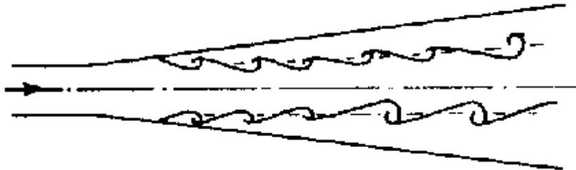
Increasing the angle of the diffuser increases the probability of boundary layer separation. In a Venturi meter it has been found that an angle of about 6 provides the optimum balance between length of meter and danger of boundary layer separation which would cause unacceptable pressure energy losses.
