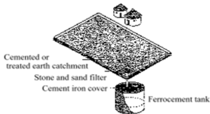
Figure 2: Ground Catchment System
